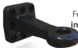
Coupling normal Ø 40 mm / 1.6" 2T
