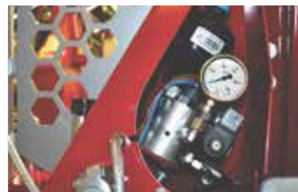
Electro hydraulic system is built into the construction and thus protected from possible damage and eather conditions.
